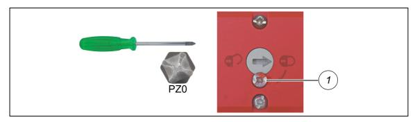
3. Turn the release dial from the locked to the unlocked position.
